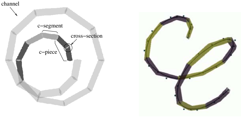
Fig. 15. Composition of a CHANNEL. ( right: ) A solution curve (control points indicated as black squares) fit into the given, transparently rendered channel whose consecutive c -pieces alternate between yellow and grey (transparent).
