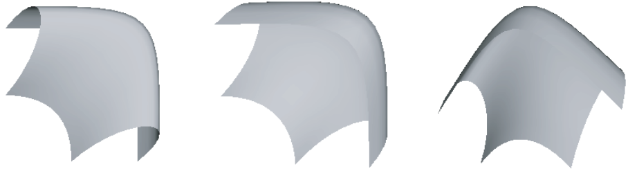
Fig. 3. Some pictures of a new surface interpolating the same Hermite curves with constant oblique tangent vectors
