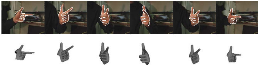
Fig. 6. Tracking a pointing hand in front of clutter. The images are shown with projected contours superimposed (top) and corresponding 3D avatar models (bottom), which are estimated using our tree-based algorithm. The hand is translating and rotating. A 2D deformable template would have problems coping with topological shape changes caused by self-occlusion.
