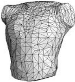
Fig. 9. Compressed star-shaped block.
