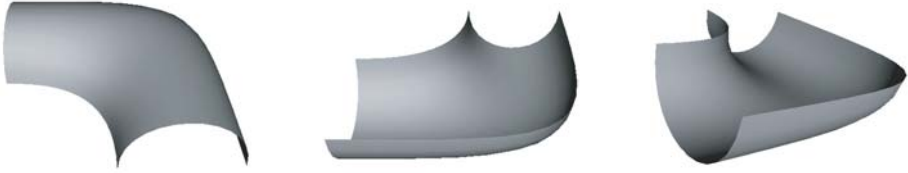
Fig. 2. Some pictures of the surface interpolating two plane Hermite curves with constant vertical tangent vectors along the curves
